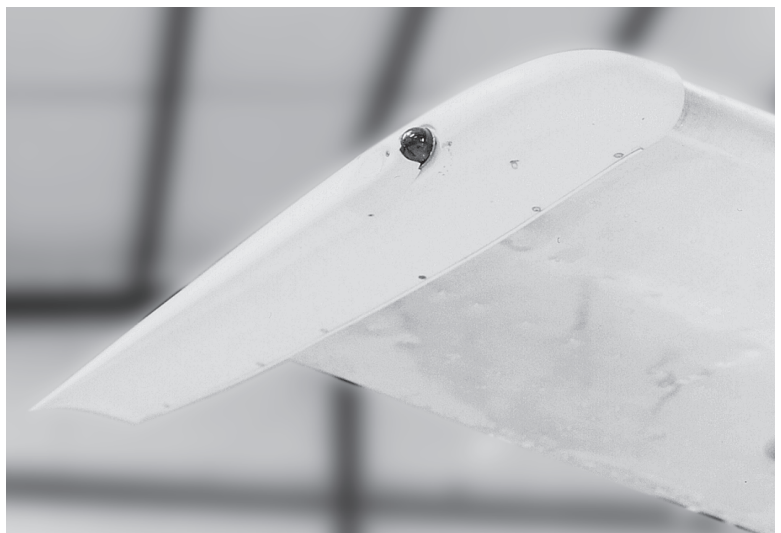
Picture showing the modern drooped wing tip installed on the wing.
